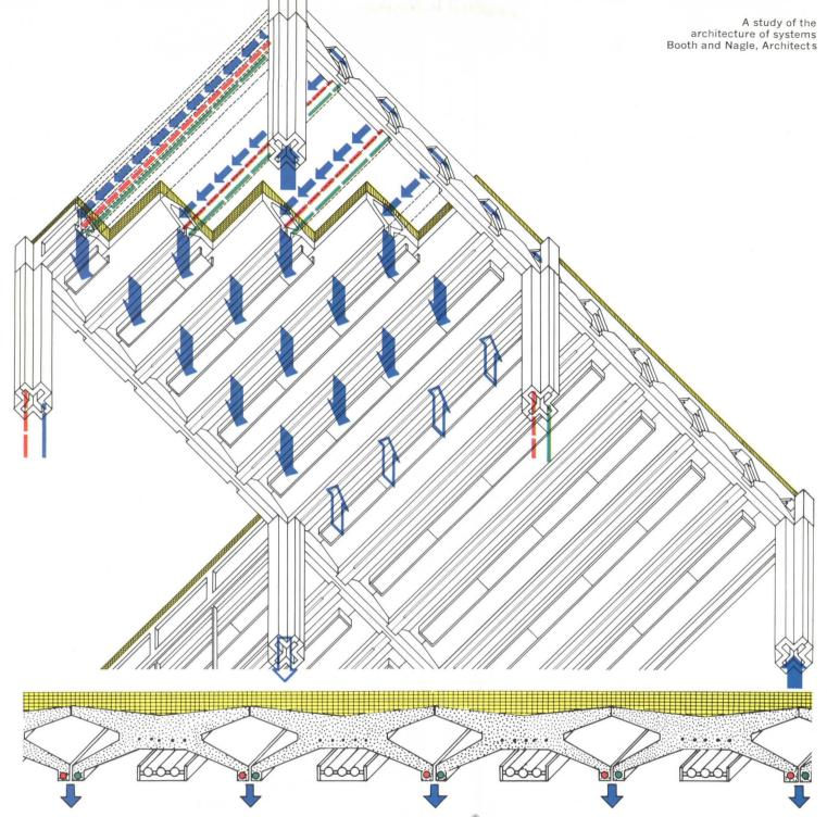
With beautiful simplicity, these pre-cast X units function as ceilings ● as plenum chambers for air supply and ⊖ return. Provide light troffers and ● power and ● communication cable raceways. ⊖ The Zonolite<sup>®</sup> lightweight concrete roof deck makes this elegant solution possible. It physically and visually unites the pre-cast sections while it insulates and protects.
