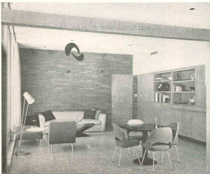
Arrangement and height of partitions in living room wing are adroitly worked out to provide for family's varying entertainment needs. Living room (above) and game room (below) can be used separately or together; ceilings are acoustically treated. Game room has door (left below) opening directly to bedroom corridor. Air conditioning ducts for this wing are in door-height cabinet (left in photo above; detail opposite)
