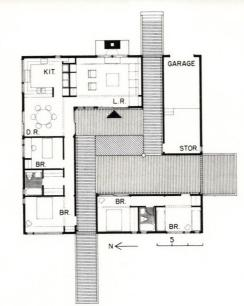
Construction is platform wood framing. Interior and exterior wall surfaces are rough-sawn cedar siding applied vertically throughout. Floors are white oak stained dark. Painted wood trim and cabinets contrast brightly with the rough-sawn cedar.
