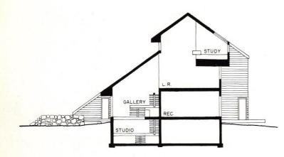
Interior walls of the Jaffe house are finished in cypress. Floors are Pennsylvania slate and pine. Major openings face east and west. The north and south elevations have limited exposures for high contrast and strong exterior shadows.
