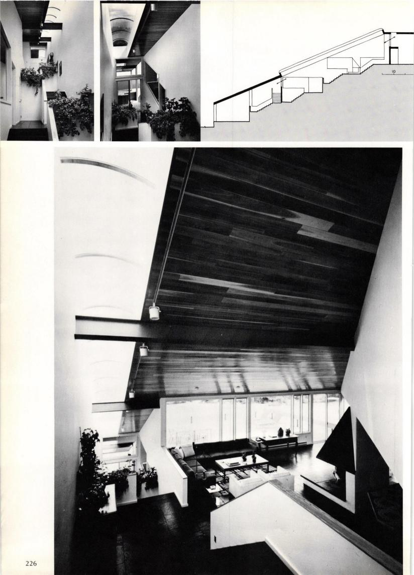
Near the entrance at the top of the house, the stairway opens directly into the living room (left), which is also seen on the right and above. The long skylight above the stairs allows solar heat generated in this space to rise to the top and exit through a large pivot window, creating a chinney effect. Outside air is drawn into the house from below, resulting in a natural air-conditioning system.
