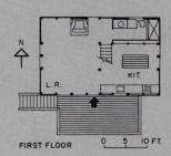
The upper level contains bedrooms with a dormitory character. The middle level, reached from the bedrooms by a stairladder, includes living, dining, kitchen and bath. The lowest level (not shown in plan) is an equipment storage area with an earthen floor.
