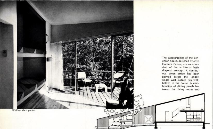
other ground floor spaces have also been painted with bands of varying widths. As panels are re-arranged in various ways, the stripes regroup to form new designs.
