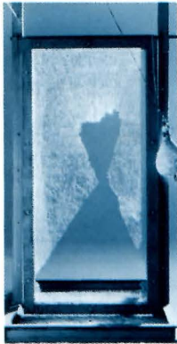
TEMPERED GLASS. This type of glass requires a higher impact energy to break. When it breaks, it shatters completely and the bag passes through it. Only a small number of glass pieces remain in the frame.
