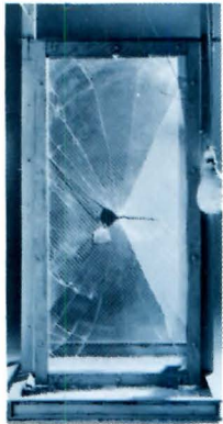
WIRED GLASS. This type of glass breaks similarly to traditional glass with the bag passing through the wire net—Shards with jagged edges surround the hole but more pieces of glass stay in place around the point of penetration. Cut wire protrudes.
