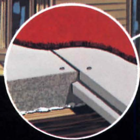
Homasote 4-way® Floor Decking for sound-deadening and resiliency: R: 3.27
