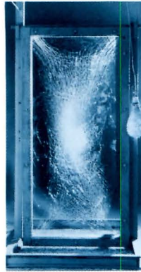
LAMINATED GLASS. Under impact, laminated safety glass is crazed but remains integral. There is no penetration of the bag. A typical cobweb pattern extends from the point of impact with the broken glass pieces adhering to the interlayer.
