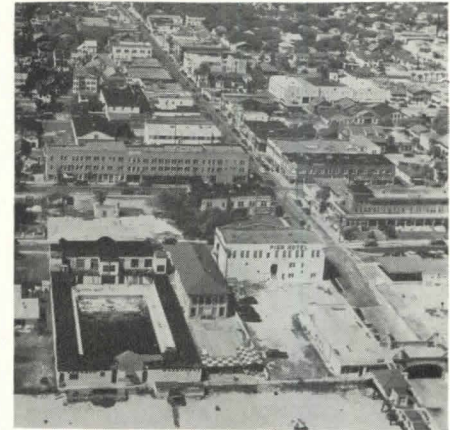
PRESENT. Main Street, but 50 feet in width (32 feet of paving), has to support two-way traffic, two curb lanes of parking, and crowds of pedestrians from the boardwalk and beach—a cluttered, noisy jumble.
