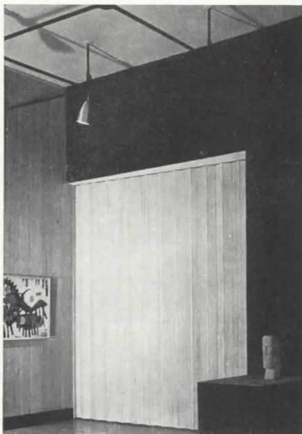
Wooden Folding Door: "Pella" / laminated-wood panels, \frac{3}{8} " thick, 3\text{-}\frac{5}{8} " wide, joined by spring hinge-fold, accordion fashion/ available in pine, oak, mahogany, or birch veneer/ may be ordered painted, clear varnished, or unfinished in custom-built or stock sizes/ Rol-screen Company, Pella, Iowa.
