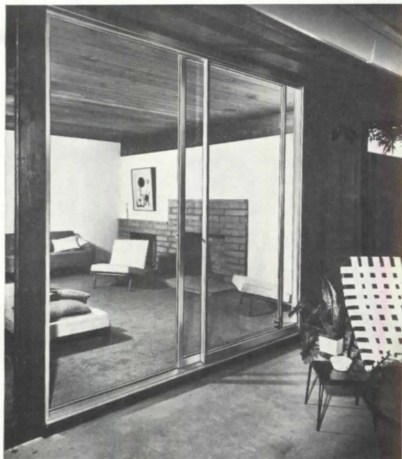
Aluminum Sliding Door: four-sided, sealed box-type aluminum extrusions/ stainless-steel roller bearings/ weatherstripped with mohair at top, interlocker, jamb, and threshold/ "Alumilite" finish provides corrosion resistance to salt air/ Ador Sales, Inc., 1631 Beverly Blvd., Los Angeles 26, Calif.
