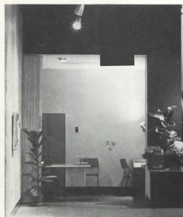
Wooden Folding Door: "Pella" / laminated-wood panels, \frac{3}{8} " thick, 3\text{-}\frac{5}{8} " wide, joined by spring hinge-fold, accordion fashion/ available in pine, oak, mahogany, or birch veneer/ may be ordered painted, clear varnished, or unfinished in custom-built or stock sizes/ Rol-screen Company, Pella, Iowa.
