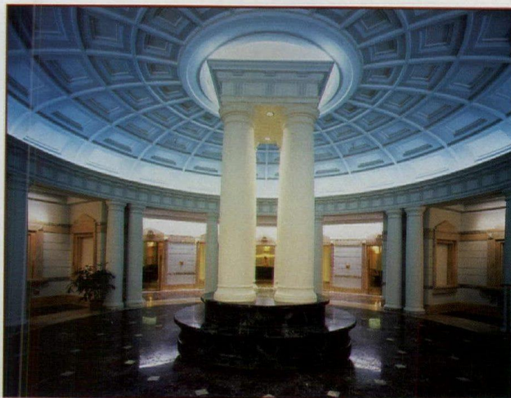
LOBBY; COFFERED CEILING BUILT OF FIBERGLASS PANELS
